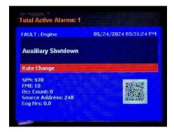
Stored Faults can be displayed by using the RABBIT and TURTLE buttons to highlight the Stored Faults icon then pressing Enter. The list shows all the controller-generated faults. The controller will also send a request to retrieve the ECU stored faults and list those as well. Alarm messages in the list are automatically removed when the alarm has not been received for a few seconds.
