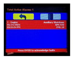
The list can be scrolled using the RABBIT and TURTLE buttons and alarms acknowledged by pressing the ENTER button, which will bring up the Alarm details. In the bottom right, is a QR-code that if scanned will take the user to the QR-Assist website for more details on the alarm (see the QR-Assist<sup>™</sup> section).
