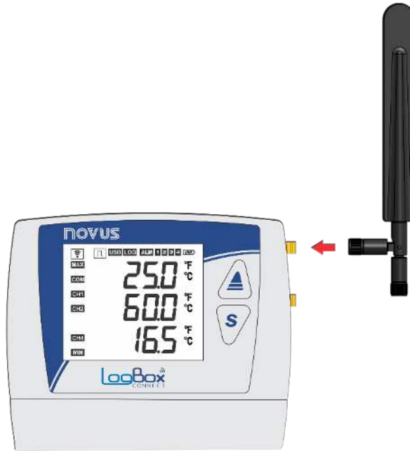
Figure 46 – Mobile network antenna
