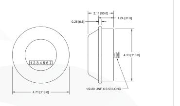
These rugged revolution counters are completely sealed, tamper resistant, and maintenance-free. They can be mounted on a rotating shaft or wheel. Adds in either direction, and records revolutions, miles, kilometers, or acres. They are used on material handling equipment, farm machinery, rapid transit vehicles, street sweepers, golf carts, and construction equipment.
