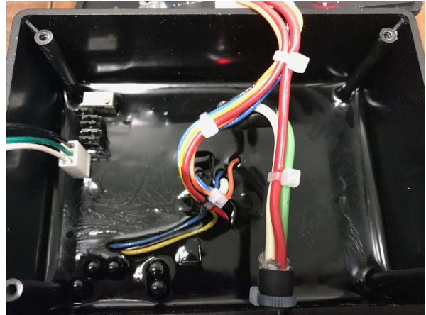
\mu VD with cover removed
