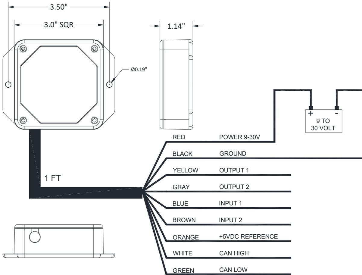
CAN Valve Driver wiring diagram
