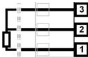
Figure 12. Input 1 - RTD Connections
